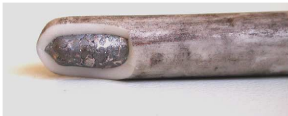
Fig. 4. Details of the Bi/Bi 2 O 3 reference electrode featured on a broken sensor.
